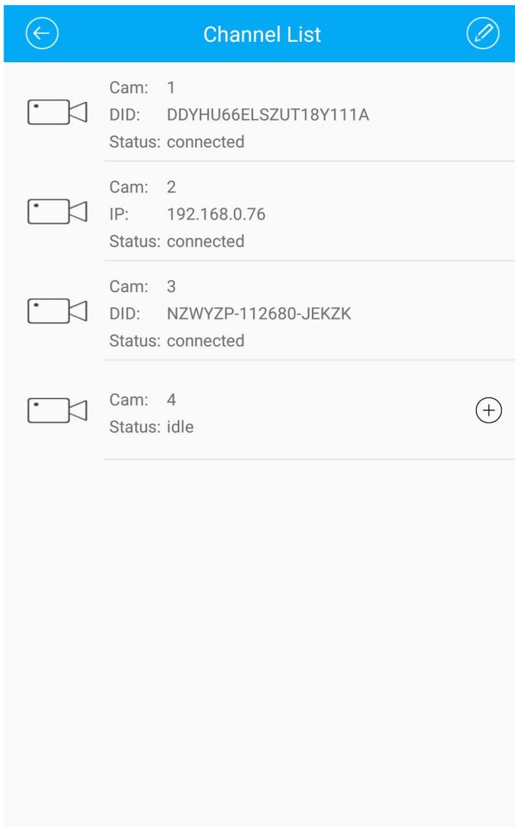
Device will show connected condition after adding, then you can add the next channel. Idle condition means no camera in the channel.
