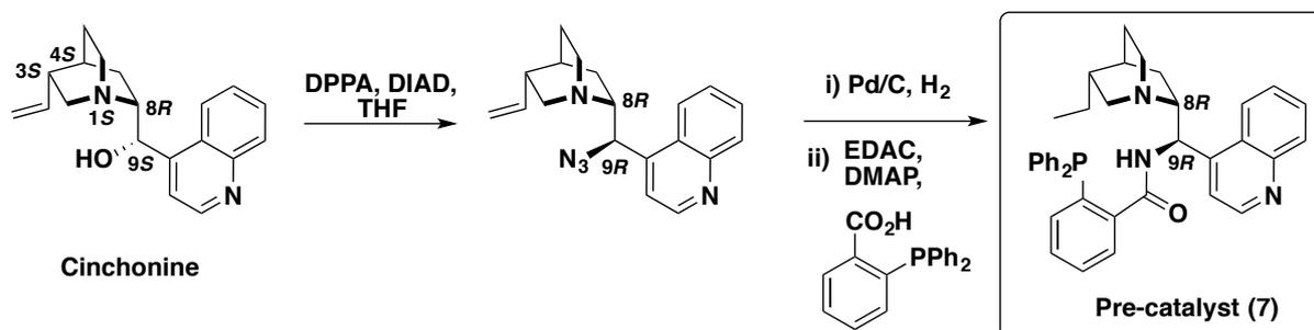
The procedures of Sladojevich *et al.*<sup>5</sup> and Cassani *et al.*<sup>6</sup> were used. Cinchonine<sup>7</sup> (3.0 g, 10.2 mmol) and triphenylphosphine (3.2 g, 12.2 mmol) were suspended in dry THF (51 ml). The mixture was cooled in an ice bath to 0°C, after which diisopropyl azodicarboxylate (2.41 ml, 12.2 mmol) was added. Diphenyl phosphoryl azide (2.64 ml, 12.2 mmol) was then dissolved in dry THF (21 ml); the resultant solution was added dropwise to the reaction mixture. Upon removing
