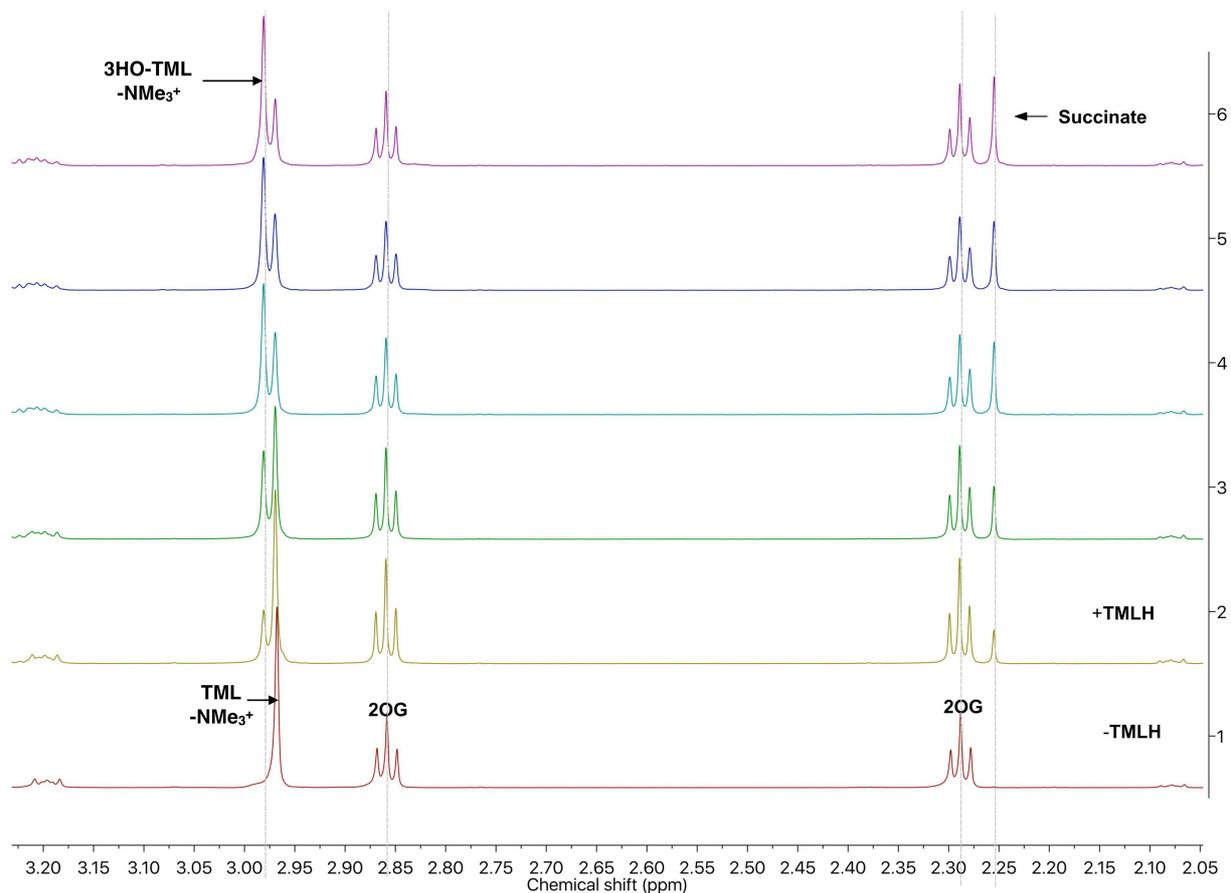
**Figure S3D** <sup>1</sup>H NMR spectra of TMLH-catalysed TML hydroxylation showing coupling of hydroxylation to conversion of 2OG to succinate, monitored over time ( $\delta = 2.05 - 3.20$  ppm). Reaction conditions: 500  $\mu$ M TML, 1500  $\mu$ M 2OG, 500  $\mu$ M *L*-ascorbate, 150  $\mu$ M Fe<sup>(II)</sup>, 10  $\mu$ M TMLH, 50 mM Tris-d<sub>11</sub>, 200 mM NaCl, pH 8.0.
