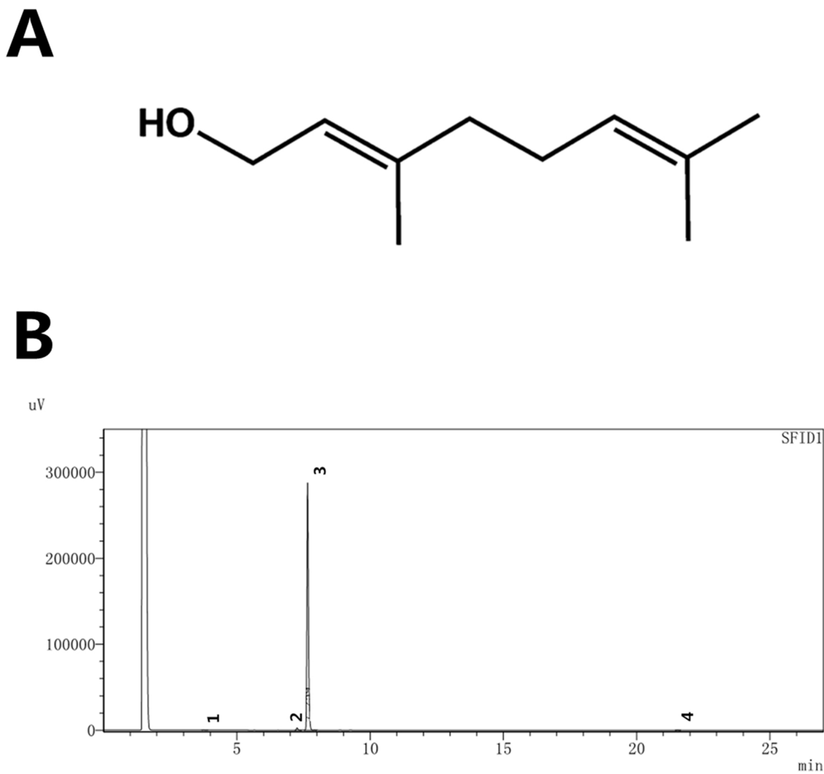
Figure 1: (A) Chemical structure of GOH, (B) HPLC chromatogram of GOH.
