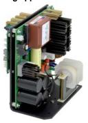
**H-Series Kit** 40 kHz @ 500 Watts Power 40 kHz @ 700 Watts Power 20 kHz @ 500 Watts Power
