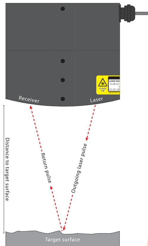
Figure 1 :: Time-of-flight measurement
