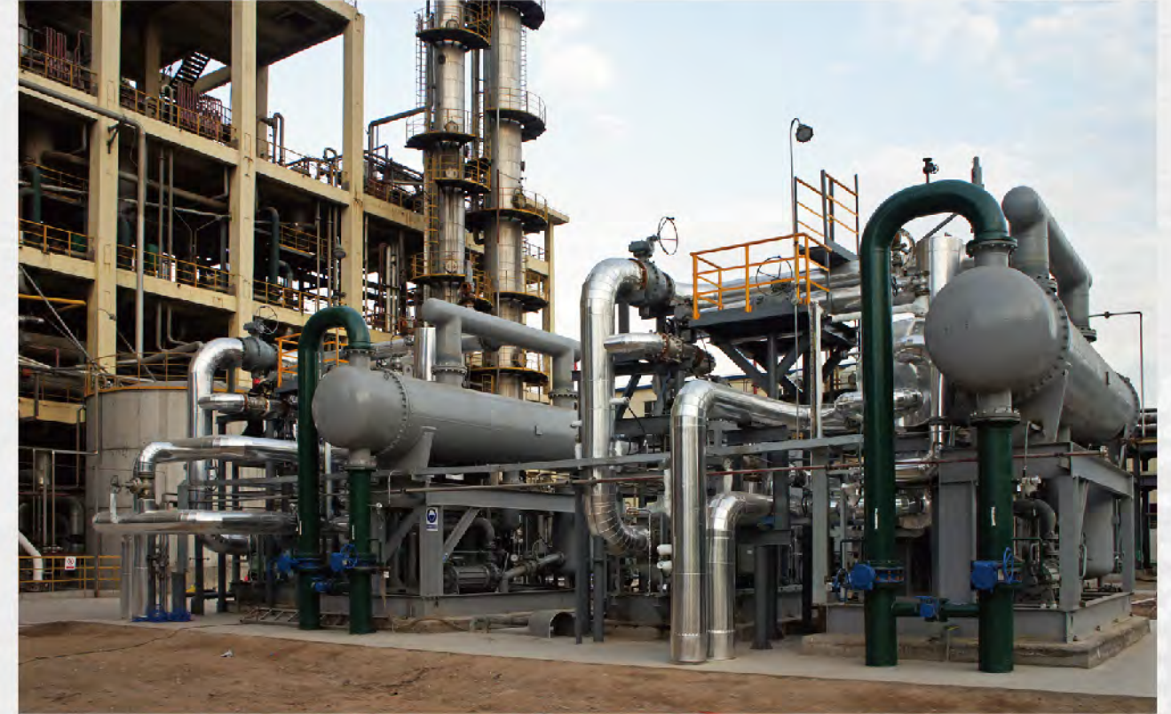
2×1200kW Hot Water ORC system (water cooled): installed in China Mainland
