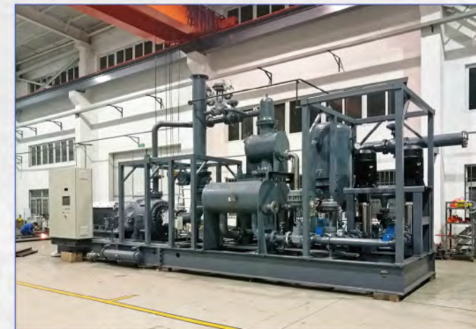
1×650kW Hot Water ORC system (air cooled): installed in China Mainland
