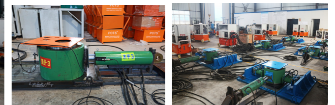
步履式顶推系统调试试验
