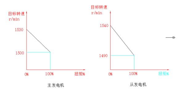
Description: Torque percentage is read in the instrument CAN message ECU, specification as per J1939. ID: 0CF00400
