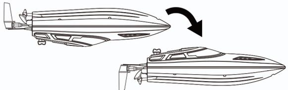
When the boat flips, press the Self-righting button, the boat can flip back.
