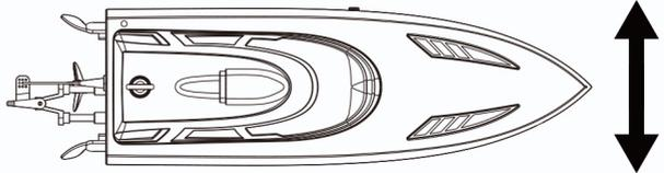
Turn the steering wheel counterclockwise and the boat will turn left; turn the steering wheel clockwise to turn right
