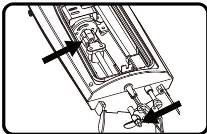
② First turn off the power and pull out the battery, then press the shaft inside the boat with one hand, and disassemble it with a wrench with the other hand
