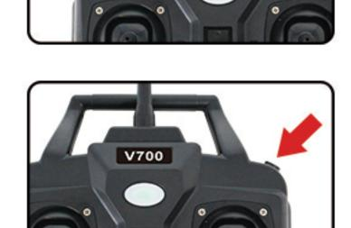
◆ Fixed-speed Cruise control: When the boat keeps moving forward, long press the fixed-speed cruise control button, the boat will enter the cruise control mode and keep going forward without remote control, remote control will continuously slowly emit "di~" and "di~" sound, and then short press fixed-speed cruise control button cancels the cruise mode. (Fixed-speed cruise control function is only available when moving forward, when the boat in low power cannot enter fixed-speed cruise
