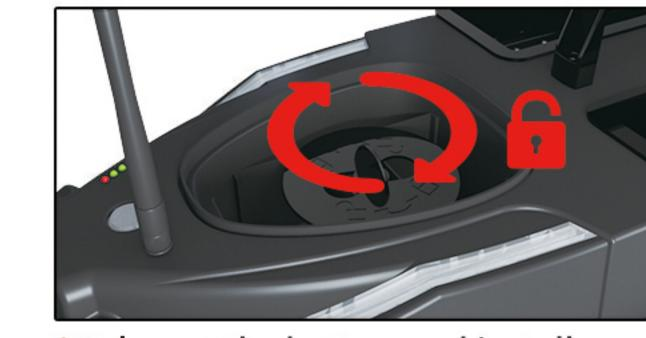
◆ Take out the battery and install Turn clockwise to open and remove the battery, press the holder into place and turn counterclockwise to secure
