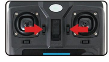
Baiting button: Press the left baiting buton to pop up the left silo, and press the right baiting button to pop up the right silo.
