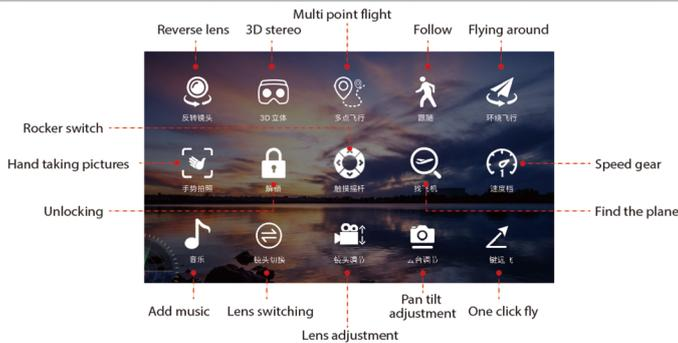
Reverse lens: rotate the lens 180 degrees.
