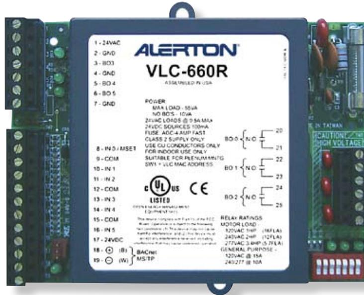
The Alerton® BACtalk® VLC-660R is a versatile, fully programmable BACnet-compliant field controller. With three software-controlled high-current relays, the VLC-660R is well suited for unit ventilator and fan-coil applications, or any application that requires multi-speed fan or motor control. As a native BACnet controller, it integrates seamlessly with your BACnet system, communicating on a BACnet MS/TP LAN at up to 76.8 Kbps.
