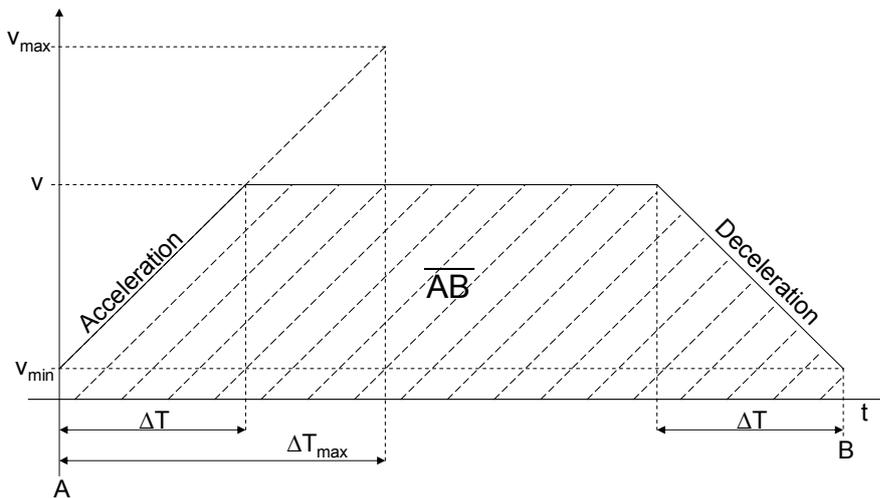
By specifying  $v_{min}$ ,  $v_{max}$ ,  $\Delta T_{max}$  and the distance from A to B, we obtain the condition for the maximum achievable velocity  $v$  and the acceleration and deceleration time  $\Delta T$ :
