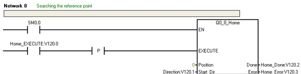
In order to explain the reference point search, the traversing diagram (Figure 4-10) is used to simulate the following case: The start position “Start” is located to the right of the reference point “Home”. The start direction “Start\_Dir” and the final direction “Final\_Dir” (+V0.2) of the reference point search are both set in negative count direction (“0”).
