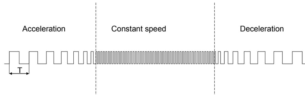
The smaller the cycle time  $T$ , the higher the travel speed.
