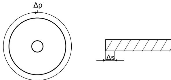
$\Delta p$  = Number of pulses required for one motor revolution
