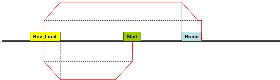
**Case B: Deceleration to "Homing\_Slow\_Spd" has not been completed before reaching the negative edge of the reference point input**
