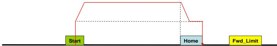
**Case B: Deceleration to "Homing\_Slow\_Spd" has not been completed before reaching the negative edge of the reference point input**
