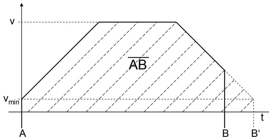
The bit „Disable\_Auto\_Stop“=“0“ (see Table 3-3) prevents that the target is passed over. The calculated target position B' is after the real target position B. If B is reached before reaching the minimum pulse frequency, the deceleration process is aborted (default setting 0). Thus a too high (late) calculation of the deceleration start point is compensated for.
