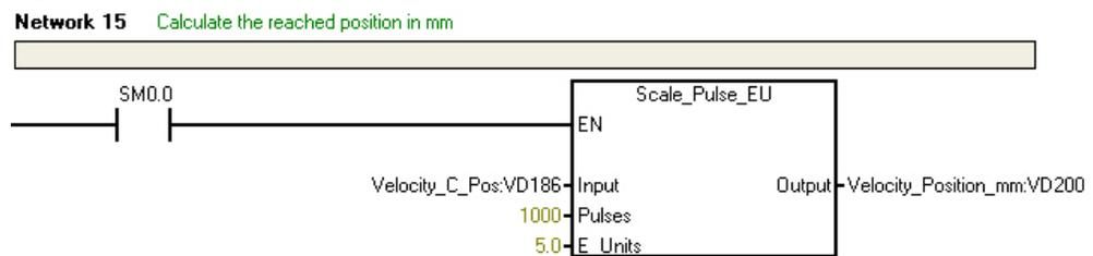
**Response** The variable "Velocity\_Position\_mm" (VD200) indicates the traveled distance in millimeters. The sign is negative due to the specified direction.
