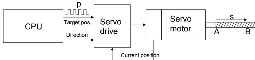
The positioning conversion from the CPU pulse output into the distance traveled by the spindle is accomplished via the reference to one motor revolution.
