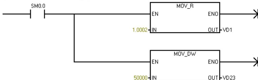
In the example, the parameter “Homing\_Fast\_Spd” (+VD23) in network 7 is set to the value “50000” pulses per second (equals the max. pulse frequency) and the “Tune\_Factor” (+VD1) is increased to 1.0002 (the deceleration ramp is started earlier).
