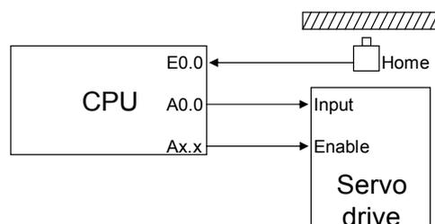
You only have to connect the servo drive to the pulse train output A0.0 and the reference point input E0.0 must be connected. It may also be necessary to enable the drive (see network 1).
