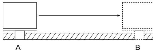
To this end, the object is accelerated to a specified speed  $v$  within the time interval  $\Delta T$ . The spindle moves with the speed  $v$ , and in order to reach the end position B, it is decelerated to zero within a second identical time interval. We obtain the distance from A to B from the area of the v-t diagram:
