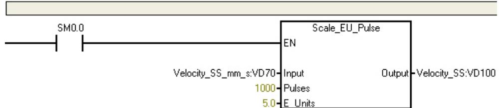
**Action** 4. Enter the value “10.0” for the variable “Velocity\_SS\_mm\_s” (VD70) (task: minimum speed of 10 mm/s) and apply the setting by clicking on
