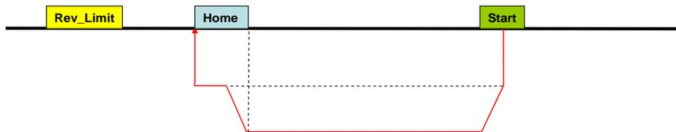
**Case B: Deceleration to “Homing\_Slow\_Spd” has not been completed before reaching the negative edge of the reference point input**
