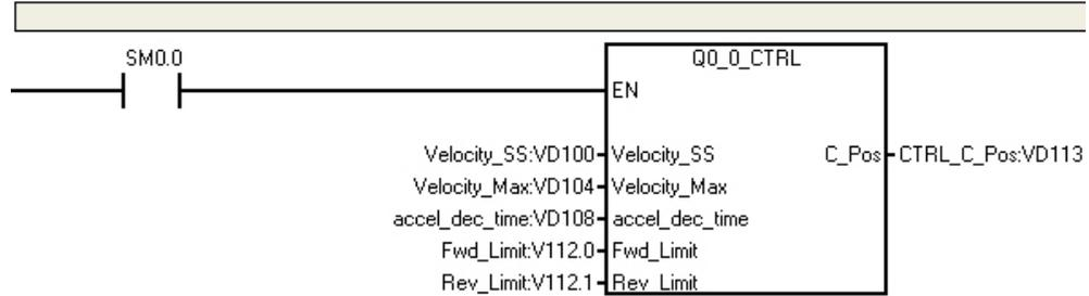
The actuation of the limit switches that limit the spindle is simulated via the variable bits V112.0 (“Fwd\_Limit”) and V112.1 (“Rev\_Limit”).
